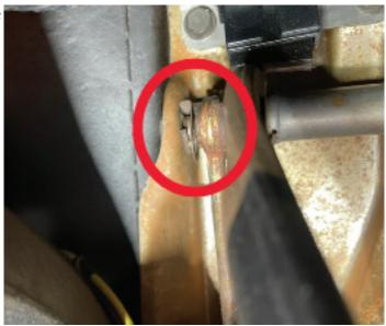
Step 3 - Use a 1/2" wrench to remove the 2 nuts that secure the master cylinder to the firewall and gently pull the master cylinder assembly out from the firewall and set
