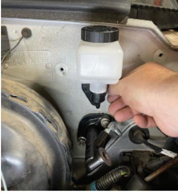
Once you have the reservoir mounted and the line connected from the reservoir to the master cylinder and also the line from the master cylinder to the bearing you are ready to fill with DOT 3 brake fluid and bleed the system. Please refer to the instructions that came with your release bearing for the proper bleeding procedure.
