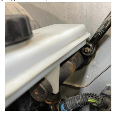
Step 4 - With the old master cylinder removed, assemble the new master cylinder assembly and ready it for installation. The new push rod uses a right and left hand threaded adjuster. For most trucks setting the distance from the center of the rod end to the master cylinder flange at 7 3/4" will achieve the correct pedal travel, but some adjustment may be necessary for your application.
