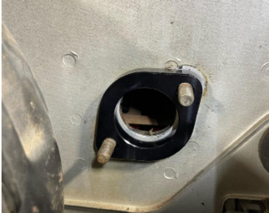
Step 8 - Slide the assembled master cylinder with push rod into the firewall opening. It will be somewhat of a tight fit, but a little extra pressure and side to side movement will get it seated enough to re-install the nuts onto the studs. Go ahead and tighten the nuts with the 1/2" wrench until snug.
