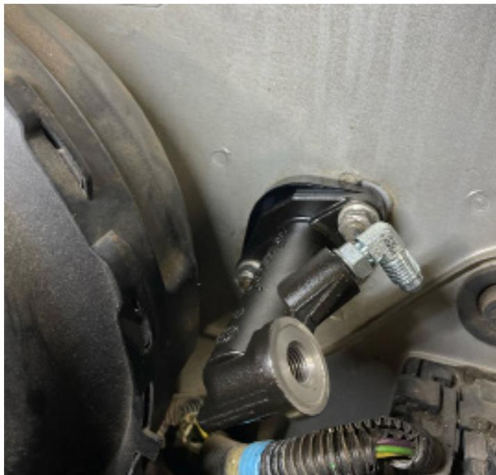
Step 9 - Once the new master cylinder has been secured to the firewall, go back under the dash and slip the rod end onto the clutch pedal pin. The plastic clip should secure it by snapping into place. At this point it will be easiest to check and make sure the push rod length adjustment is set correctly.
