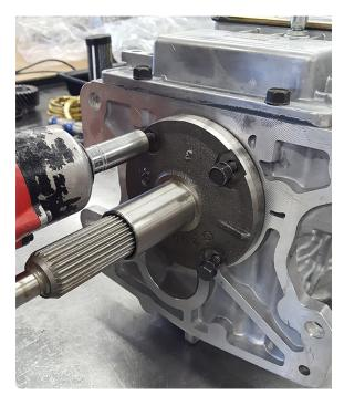
Once the Tremec retainer has been removed check for the input shaft bearing race and bearing shims. Sometimes they will stick to the backside of the Tremec retainer. It is imperative that these are transferred to the new Tilton retainer.
