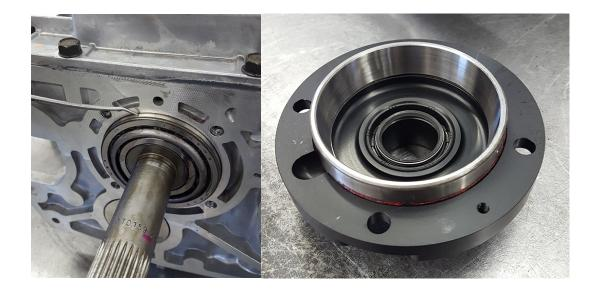
Before bolting the Tilton retainer on, be sure to add some RTV sealant to the sealing surface of the retainer and spread it evenly across the mounting surface. Use the sealant sparingly as you want to avoid excessive sealant pressing into the transmission.
