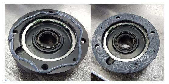
Slide the new Tilton bearing retainer over the input shaft and re-install the 4 original Tremec bolts to secure it to the transmission case. Torque the bolts to 15 ft/lbs.
