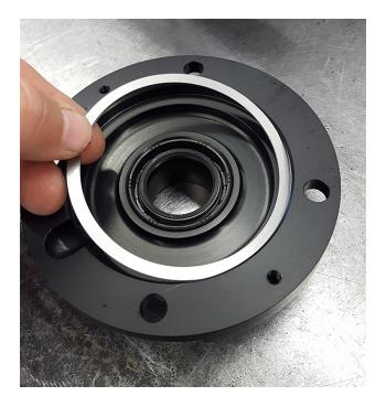
The bearing race can be put into the case or into the back of the new Tilton retainer for reinstallation.
