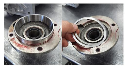
Thoroughly clean the bearing race and transmission case surface to ensure no residual red sealant is remaining on those parts. Then transfer all the bearing shims to the Tilton retainer. Each TKO is shimmed individually, so there may be one or several shims, the important step is to make sure all shims that were in there when the Tremec retainer was removed are transferred.
