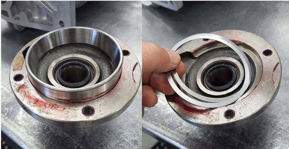
Thoroughly clean the bearing race and transmission case surface to ensure no residual red sealant is remaining on those parts. Then transfer all the bearing shims to the Tilton retainer. Each TKO is shimmed individually, so there may be one or several shims, the important step is to make sure all shims that were in there when the Tremec retainer was removed are transferred.
