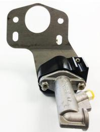
• Install master cylinder with plate by sliding the rod end linkage through the opening in the firewall where the original clutch rod was located. The mounting plate will locate on the studs that attach the brake master cylinder to the firewall; you can then reattach the brake master cylinder and tighten all fasteners.
