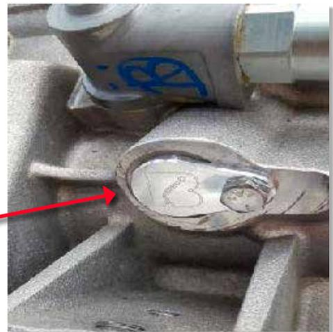
The epoxy sealed control module should be attached to the transmission using the bolt that fastens the speed sensor clamp. Do not overtighten this bolt.
