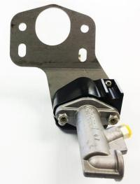
• Install master cylinder with plate by sliding the rod end linkage through the opening in the firewall where the original clutch rod was located. The mounting plate will locate on the studs that attach the brake master cylinder to the firewall; you can then reattach the brake master cylinder and tighten all fasteners.
