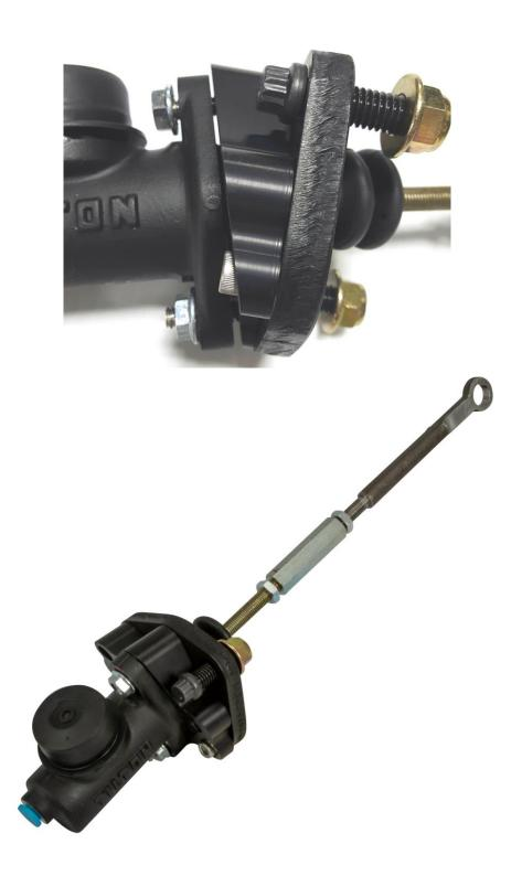
• Install master cylinder with plate by sliding the rod end linkage through the opening in the firewall where the original clutch rod was located. The mounting plate will be secured to the firewall using the supplied hardware.
