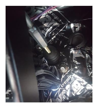
• Install the new adjustable pushrod onto the stud of the clutch pedal and secure with the clip pin.
