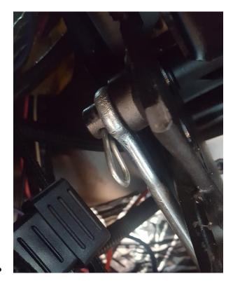
• The rod-end and linkage will need to be set to the length that gives you the correct height for your clutch pedal. It can be lengthened or shortened to get the desired pedal height. If adjustments are made, make sure there are at least 5 full threads penetrating the rod end.
