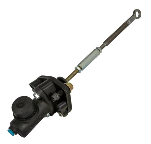
• Install master cylinder with plate by sliding the rod end linkage through the opening in the firewall where the original clutch rod was located. The mounting plate will be secured to the firewall using the supplied hardware.
