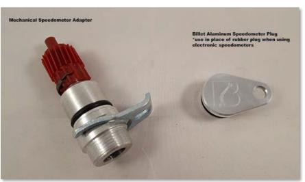
If you will be utilizing a mechanical speedometer we can equip your Tremec with one of our cable adapters. We will just need to get your rear gear ratio and rear tire size to set the adapter up with the proper gear. If you will be using an electronic speedometer or not using the mechanical speedometer, then you will need to replace the rubber plug with our billet speedo plug. This will ensure you do not experience any fluid leaks from the rubber plug coming loose or falling out completely.
