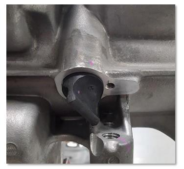
Factory installed rubber plug. This is where the mechanical speedometer pick up is located. You will need to replace this rubber plug with either our billet speedo plug or a mechanical cable adapter. Both are listed below should you still need one or the other please give us a call. 618-943-4856
