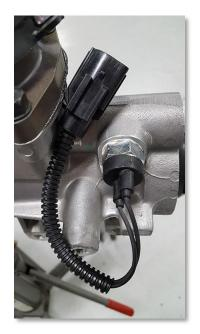
TKO Neutral Safety Switch- Optional to use. There is currently no pigtail adapter available. If you choose to use it, just clip the attached connector off and hard wire it into your starter solenoid power wire.
