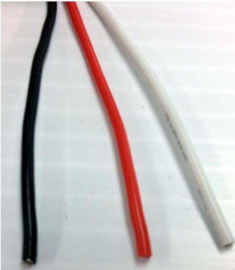
The **Red** wire should be connected to a fused +12 volt ignition switched or constant power supply.
