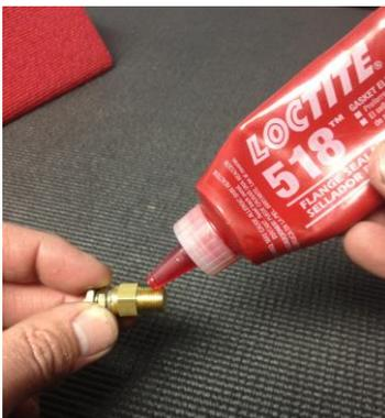
**Sealant applied to sensor**
