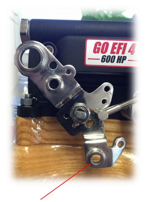
To determine if our Tru-shift system will fit your FITech system we need the outside diameter of the lower mount hole please. If the raised boss is .375''(+/-.005'') we have a kit. If the raised boss is .455''(+/-.005'') we do not have a kit.
